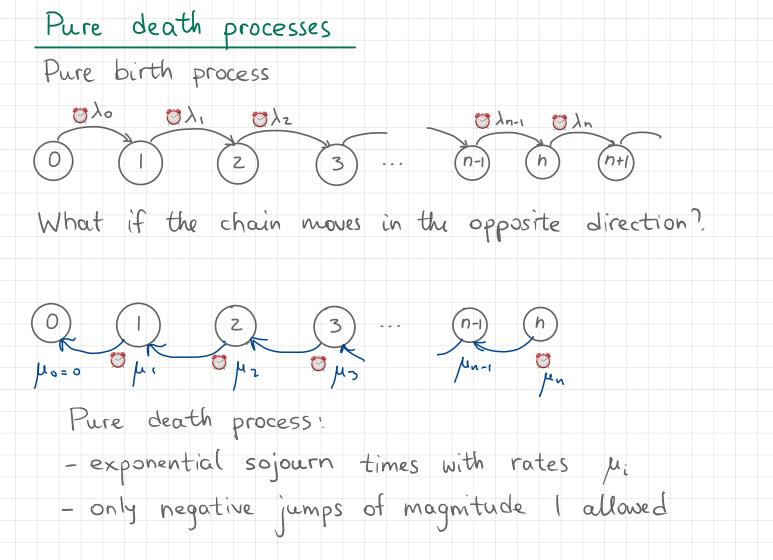
Pure death processes Infinitesimal description: Pure death process (X+)+20 of rates (µk)k=1 is a continuous time MC taking values in {0,1,2,--, N-1,N} (state O is absorbing) with stationary infinitesimal transition probability functions (a) Pk, K-1 (h) = Mk h + O(h), K=1,-1, N  $h \rightarrow 0$ (b) PKK (h) = 1-M. h+o(h), K=1, ..., N (c) Pkj (h) = 0 for j>k. State 0 is absorbing ( uo=0)
