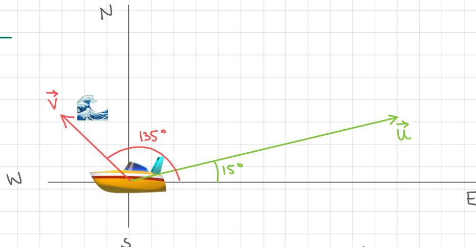
Ship travels  $15^\circ$  north of east with engine generating a speed of 20 knots in this direction. The ocean current moves the ship NW at a speed of 2 knots. How much does the current slow the movement of the ship in the direction of  $\vec{u}$ .
