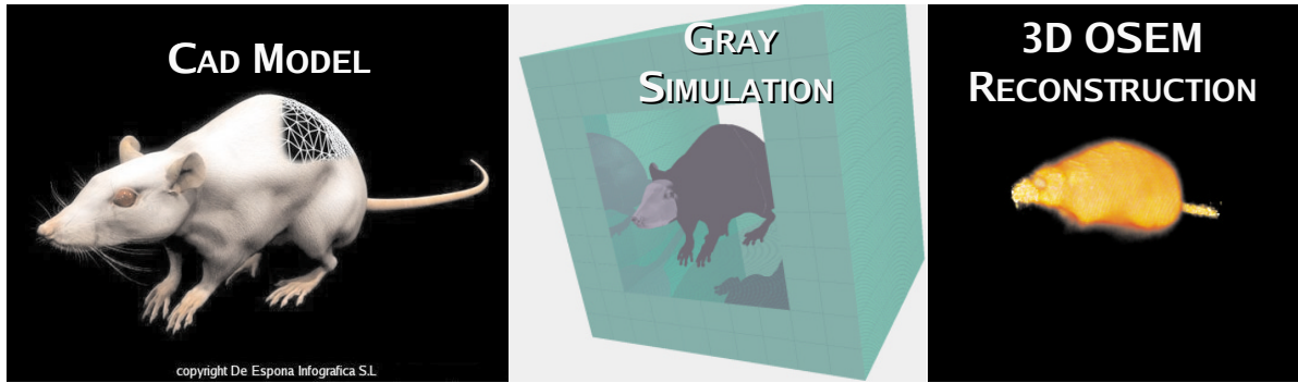
Fig. 2. The complete path from source geometry through image reconstruction: Detailed 3-D CAD modeling of a rat phantom (LEFT), import of the vector geometry into GRAY to generate a simulated scan of a uniform distribution of positron decays in a rat placed in a 1mm resolution small animal box LSO-PSAPD PET scanner (MIDDLE), and a volumetric visualization of a reconstruction of the rat using a fully 3-D list-mode OSEM image reconstruction (RIGHT).
