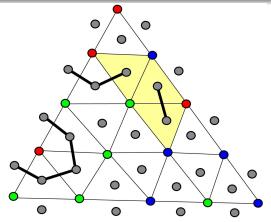
For an "R-G" path: feasible triangles are ones with both Red and Green. Outgoing direction keeps Red to the left and Green to the right. Initially at outer left triangle. All other sources/sinks are panchromatic triangles.
