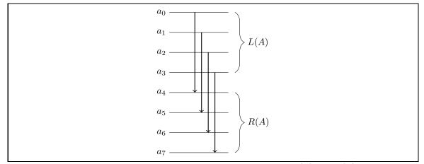
Figure 3: A single layer sorting network to compute L(A) and R(A)
