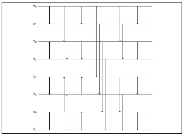
Figure 2: BatcherSort for 8 inputs
