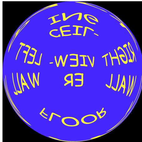
Figure VI.10: An environment map mapped into a sphere projection. This is the kind of environment map supported by OpenGL. See color plate C.7. The scene is the same as is shown in Figure VI.11. Note that the front wall has the most fidelity, and the back wall the least. For this reason, spherical environment maps are best used when the view direction is close to the direction used to create the environment map.
