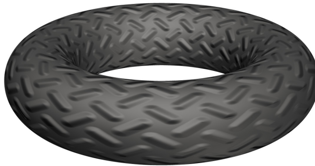
Color Plate C.6: (Figure VI.8, page 207.) A bump mapped torus. Note the lack of bumps on the silhouette. There are four white lights shining on the scene, plus a low level of ambient illumination. This picture was generated with the ray tracing software described in Appendix B.
