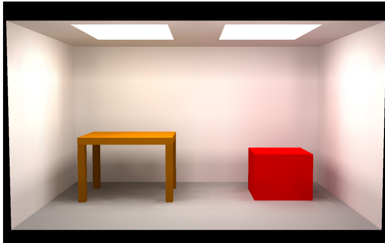
Color Plate C.15: (Figure XII.3, page 399.) A radiosity rendered figure, with smooth shading of illumination. The red color of the box is reflected onto the nearby walls, giving them a slight reddish hue. This is based on the patches shown in Figure XII.1.
