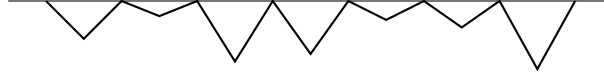
Figure IV.19: For the derivation of the geometric term, G , the microfacets are modeled as symmetric, “V”-shaped grooves with the tops of the grooves all at the same height. The horizontal line shows the overall plane of the surface.
