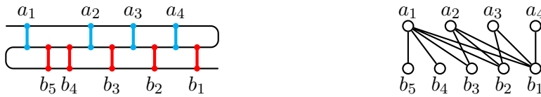
Figure 11: An example of a graph that can be formed with two folds.
