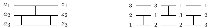
Figure 8.2 Left: A sorting network with inputs a_i and outputs z_i . Vertical lines are comparators Right: What the network does to the inputs 3,2,1.
