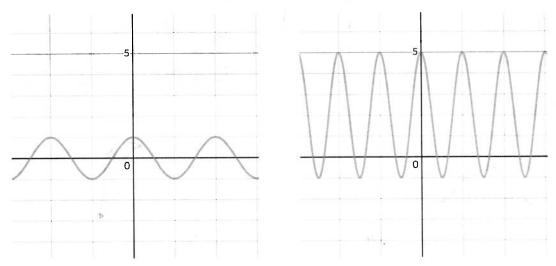
To transform the left graph into the right graph, the amplitude has been tripled, the period has shrunk by a factor of two, and the graph has been shifted up by 2 units.
